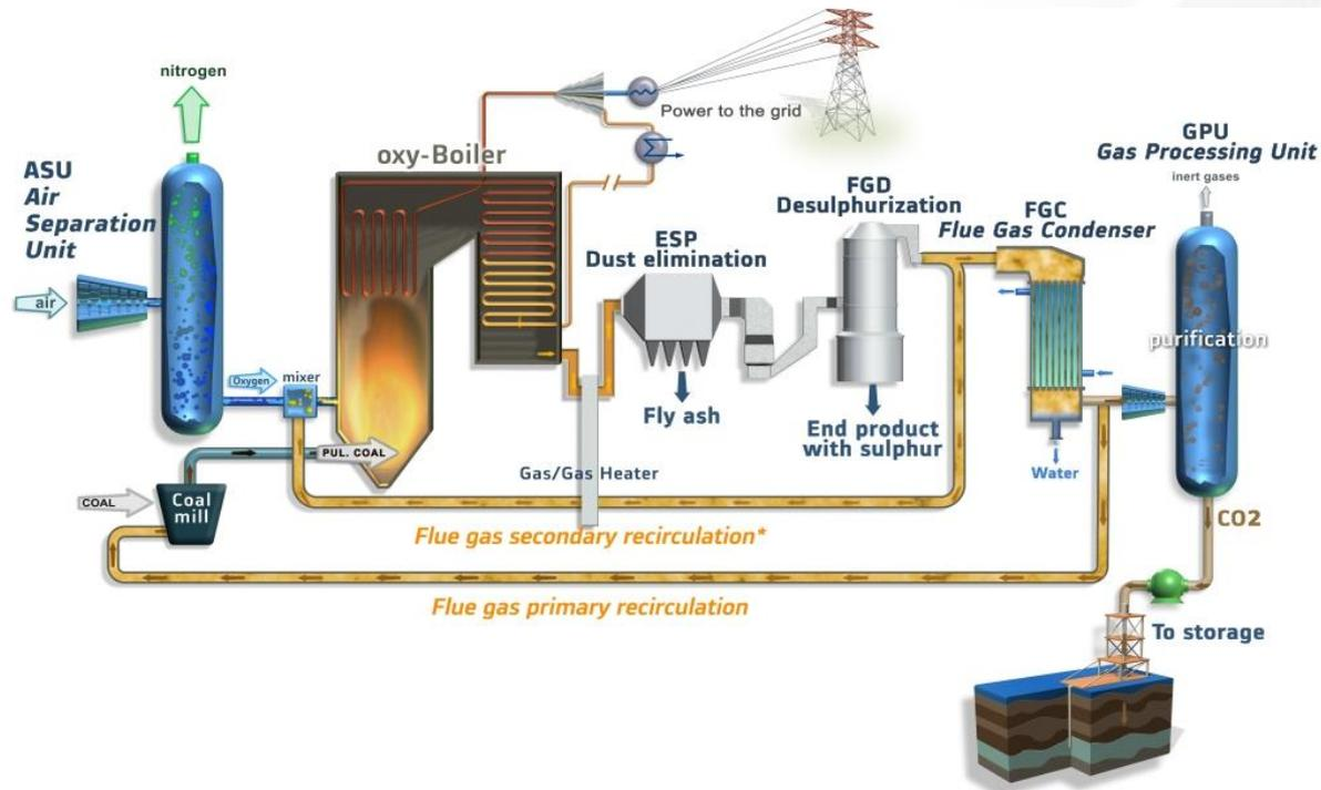
Oxy-combustion technology already validated at pilot scale
